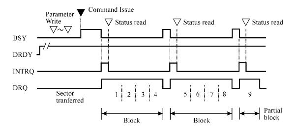
Figure 5.2 Execution example of READ MULTIPLE command
